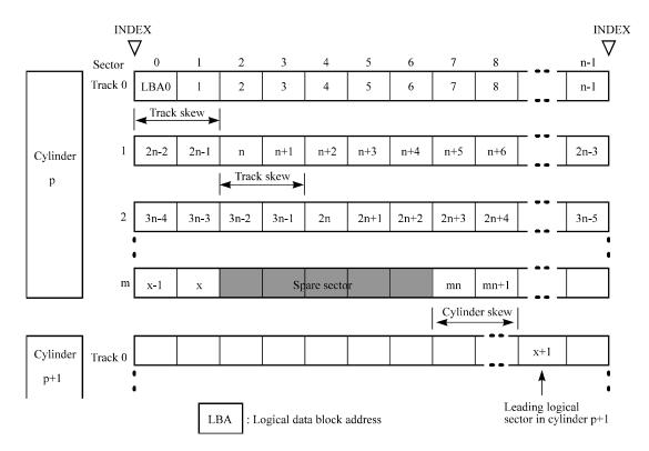
Figure 3.5 Track skew/cylinder skew
